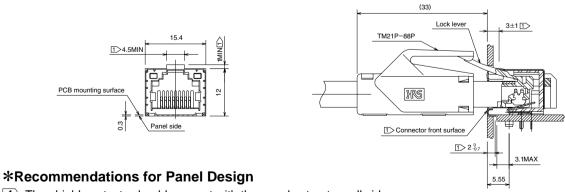
1 The shield contacts should connect with the panel cut-out on all sides.
