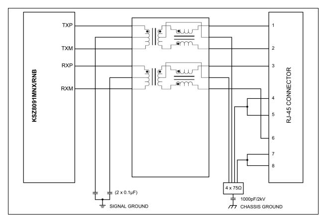
FIGURE 11-1: TYPICAL MAGNETIC INTERFACE CIRCUIT
