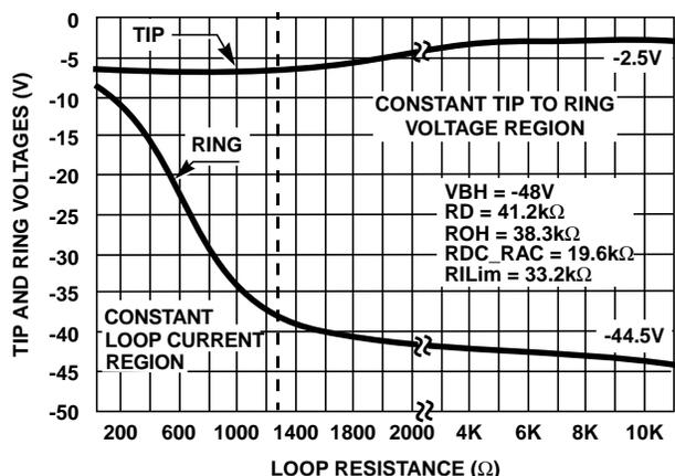
FIGURE 2. TIP AND RING VOLTAGES vs LOOP RESISTANCE
