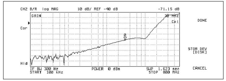
**Figure 2. Off Isolation vs Frequency**
