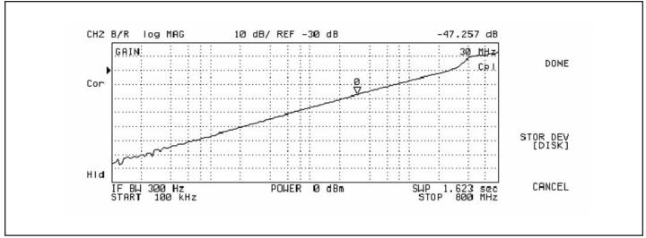
Figure 3. Crosstalk vs Frequency
